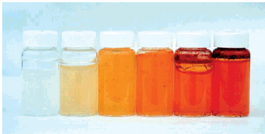
Figure 3. Decavanadate-incorporated silica gels of various vanadium concentrations after aging at 86 °C for 18 h. Samples are VSi0.0, VSi2.3, VSi4.4, VSi19, VSi32, and VSi48 from left to right.
